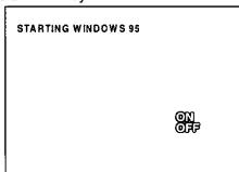
Windows 95 start up menu will be displayed. Then select "Safe mode" by using down arrow key or type in the number.
